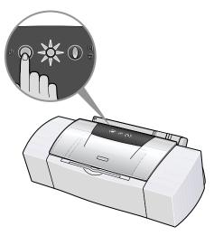
**Note** If the POWER lamp changes to orange and begins flashing, refer to the section "**Handling Error Messages**" on page 55.
